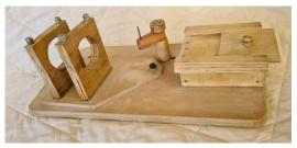
and the jig suits all blade sizes. With an angle grinder with a diamond disc attached Trevor is now sharpening away. The MDF was left raw ( no finish) and the angle grinder has been omitted in these photos for clarity.
