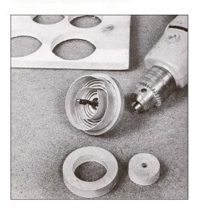
When you need small wood rings use two blades simultaneously in the hole saw.
